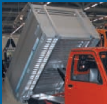
The renowned aluminium flatbed bodies from PWP in building block system. Can also be supplied as tipper.
