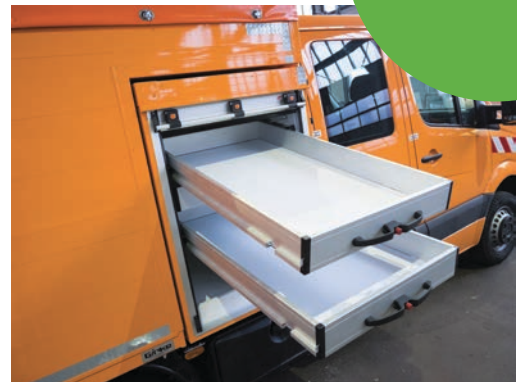
Drawers linearly or pivotally downwardly extendable
